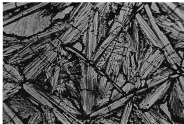
Figure 5. Microstructure of eutectic I of 2,4-dinitrophenol (1) + naphthalene (2) \times 150 .
