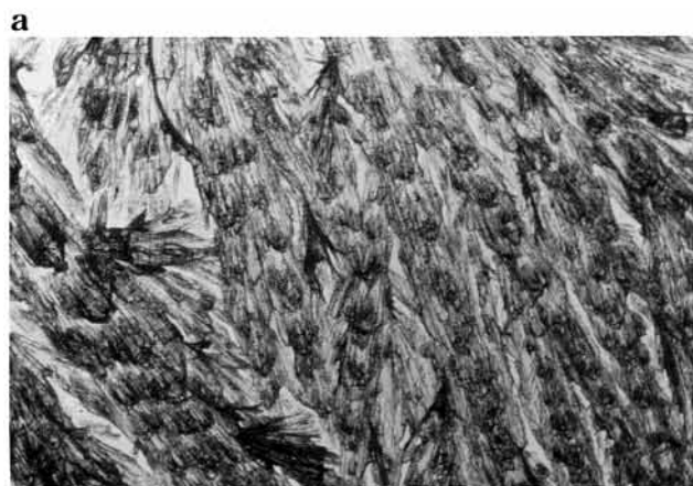
Figure 5. Microstructure of eutectic I of 2,4-dinitrophenol (1) + naphthalene (2) \times 150 .
