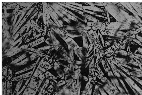
Figure 6. Microstructure of eutectic II of 2,4-dinitrophenol (1) + naphthalene (2) \times 150 .
