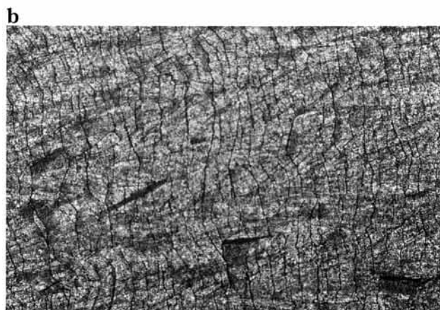
Figure 6. Microstructure of eutectic II of 2,4-dinitrophenol (1) + naphthalene (2) \times 150 .
